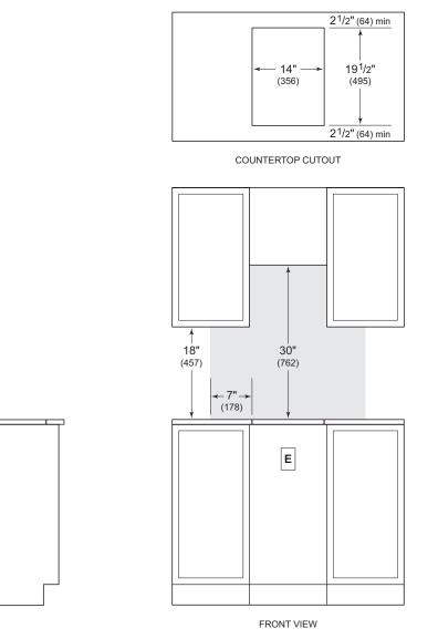
NOTE: Shaded area above countertop indicates minimum clearance to combustible surfaces, combustible materials cannot be located within this area.
