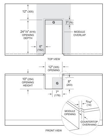
NOTE: Shaded area above countertop indicates minimum clearance to combustible surfaces, combustible materials cannot be located within this area. An insulating liner is not required.
